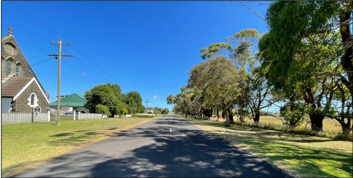
Figure 9 - surrounding existing road network features 30m widths, with 10m+ grassed nature strips, swale drains and intermittent street tree plantings – looking south along Horne Street, with subject land on right.
