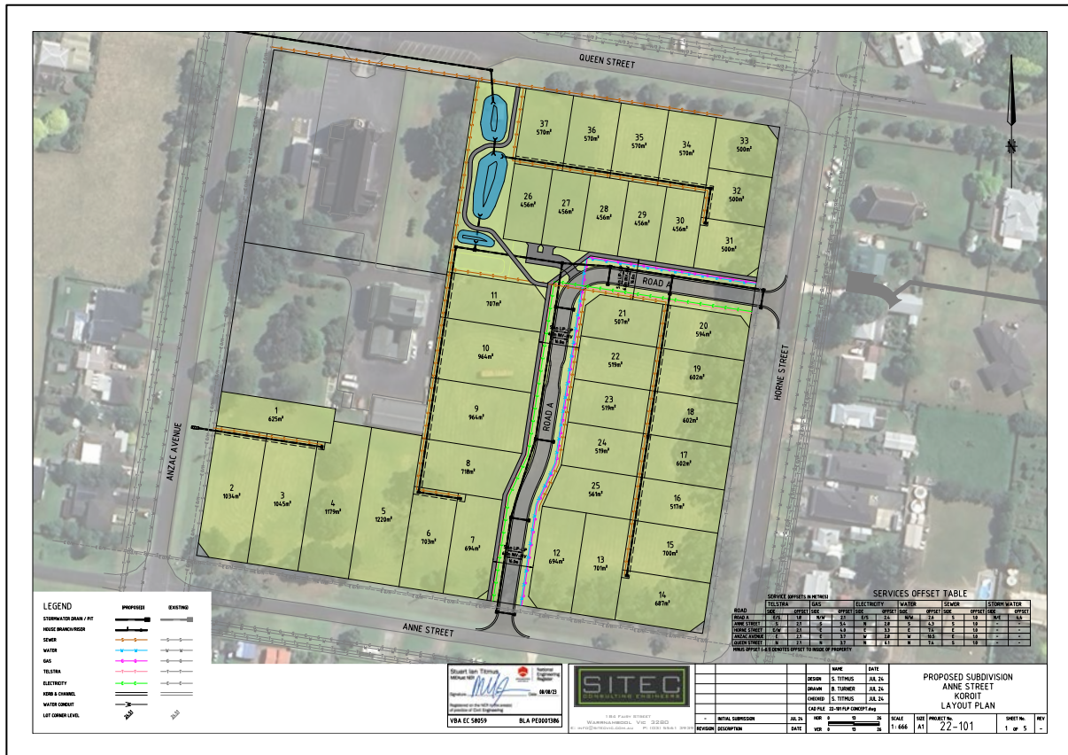
Figure 1 Proposed plan of subdivision – shown with proposed internal servicing mains location (does not detail individual lot connections)
