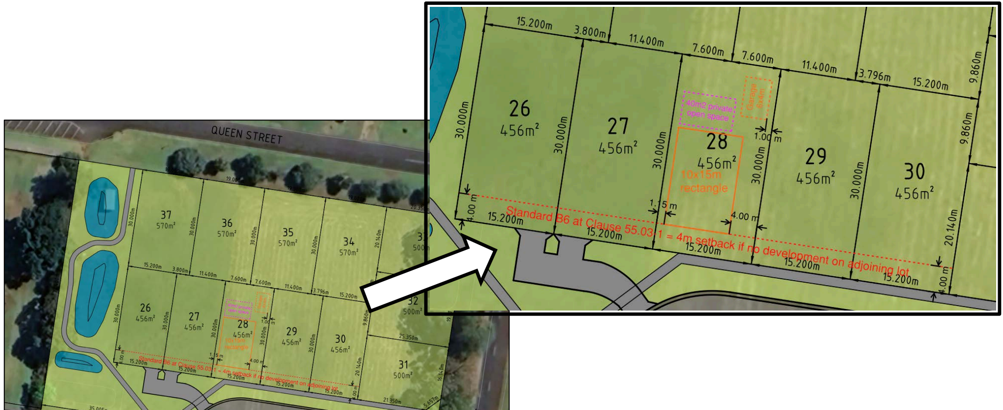
Figure 18 - 10x15m rectangle, 4m front setback, 4m driveway, side setback, 6x4m garage and 40m 2 lot capacity on smallest lots. Standard for lot capacity for future development met.
