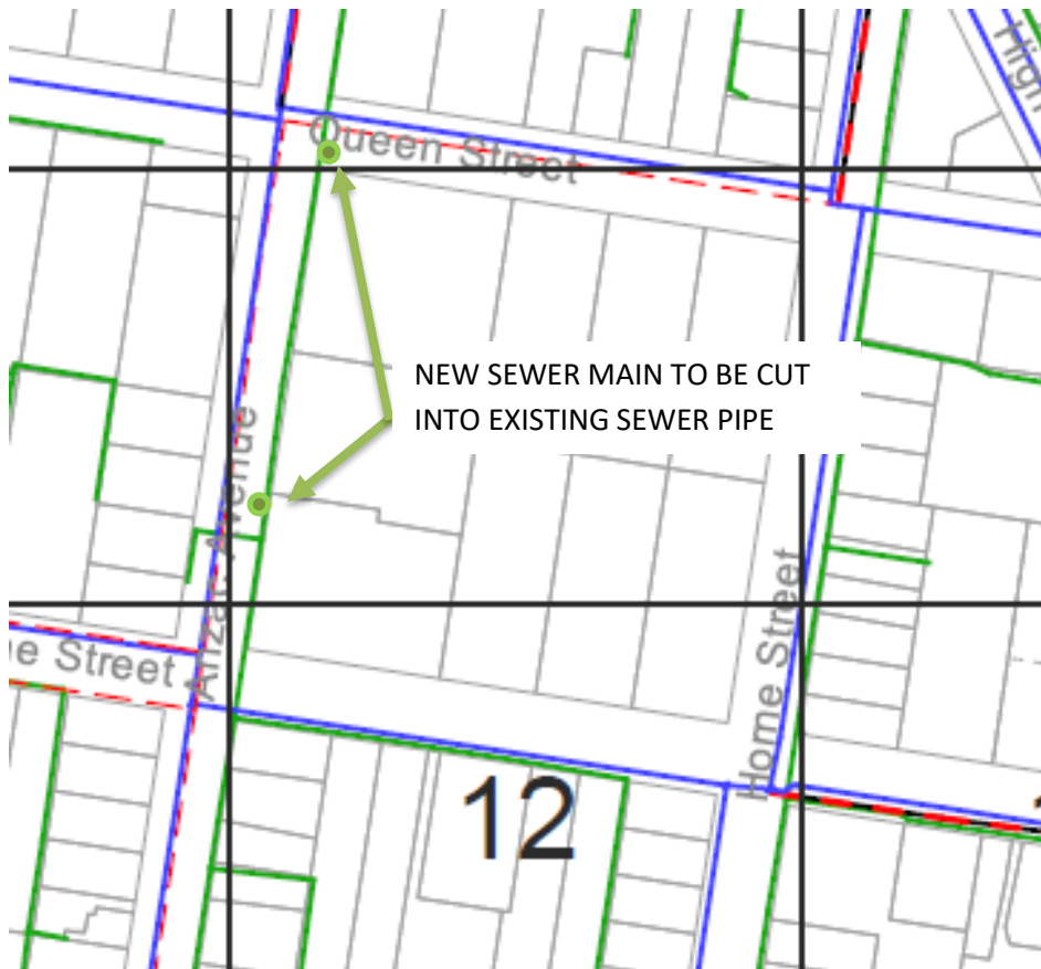
FIGURE 6: POSSIBLE SEWER RETICULATION CONNECTION POINTS
