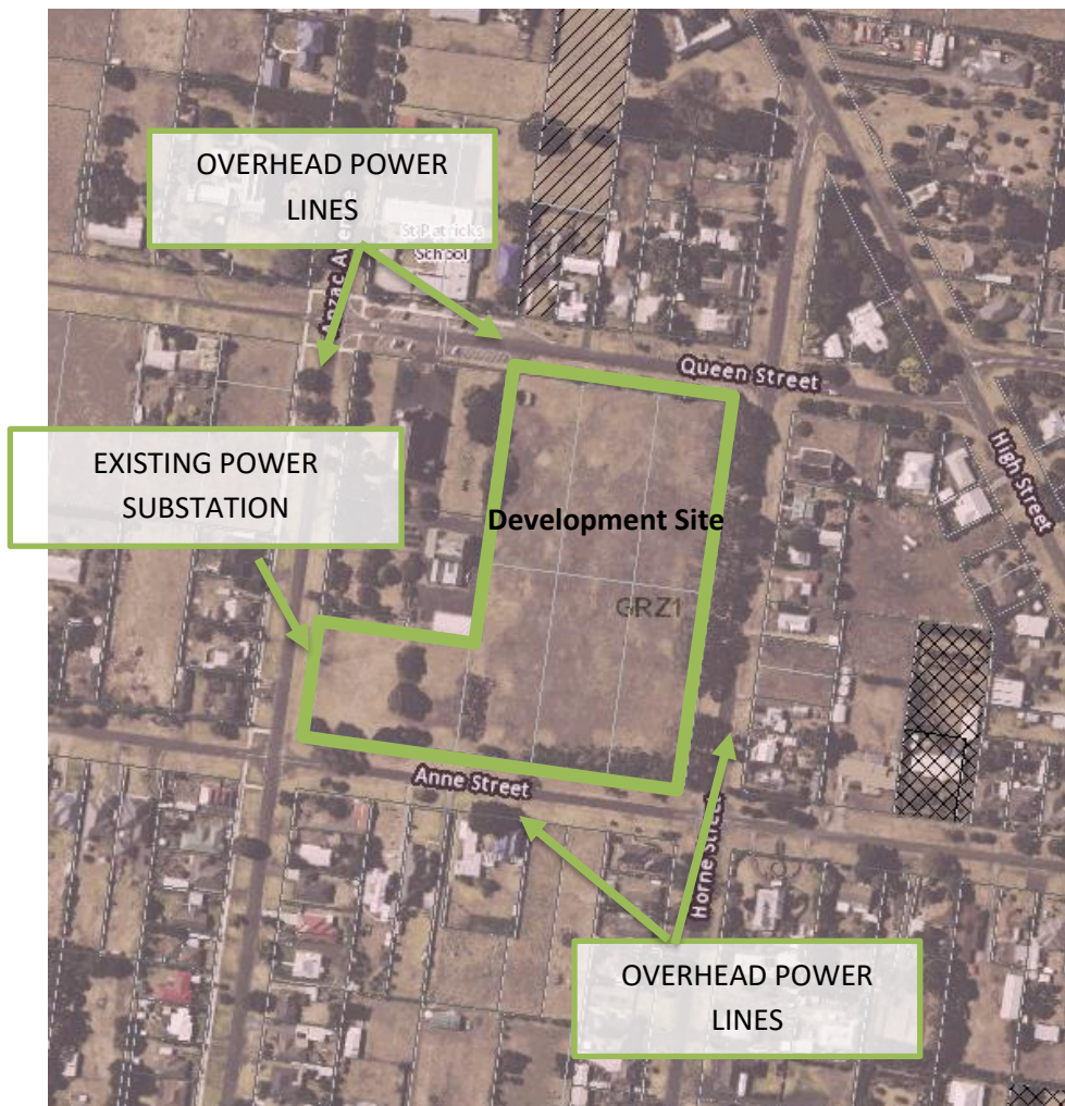
FIGURE 10: POWER CONNECTION POINTS
