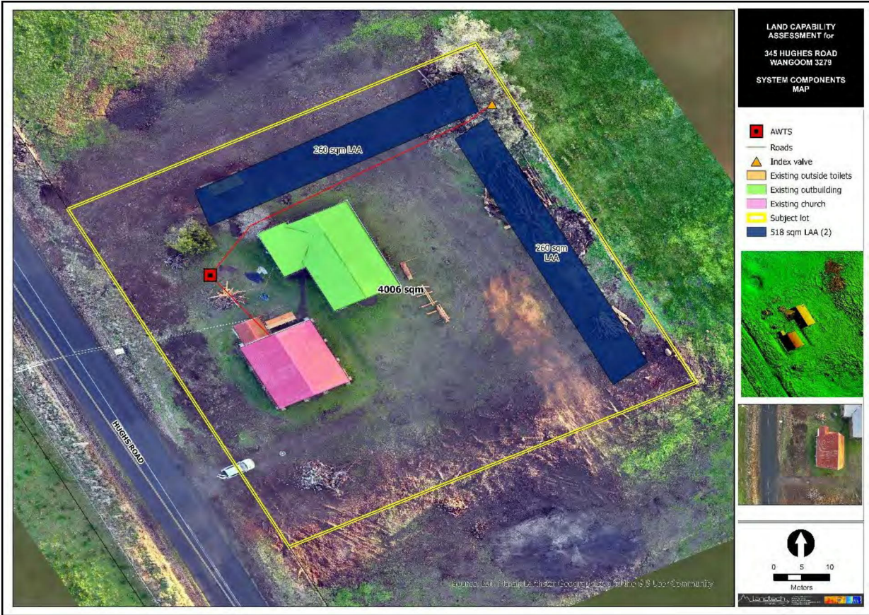
Figure 27 – Secondary treatment option using subsurface irrigation for disposal with split fields and increased flexibility.
