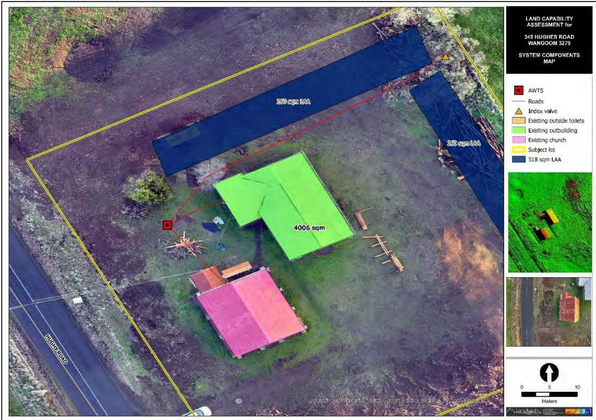
Figure 28 – Closer view of secondary treatment option using subsurface irrigation for disposal with split fields and increased flexibility.
