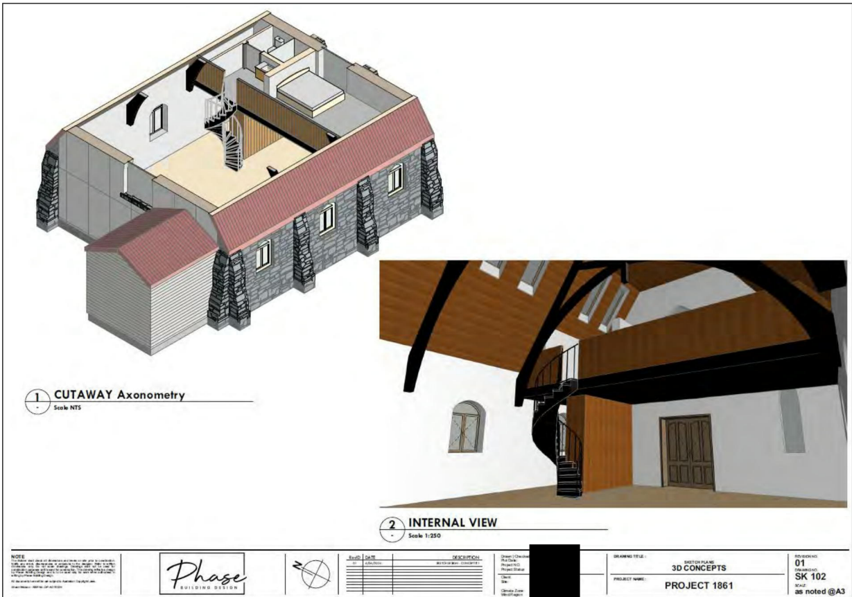
Figure 10 – Internal church renovation detail (Source: Phase Building Design 2024).
