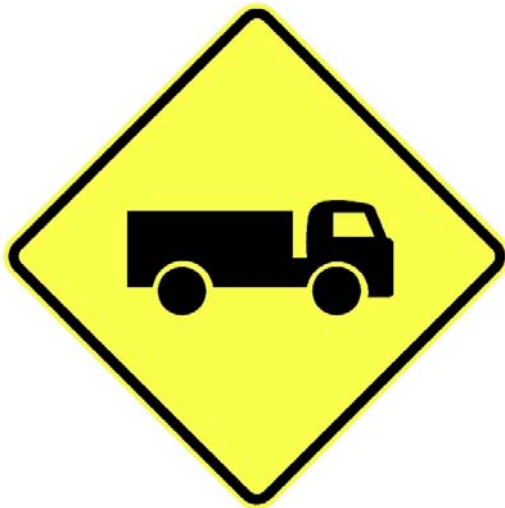
WARNING SIGN W5-22 – TRUCK SYMBOLIC
