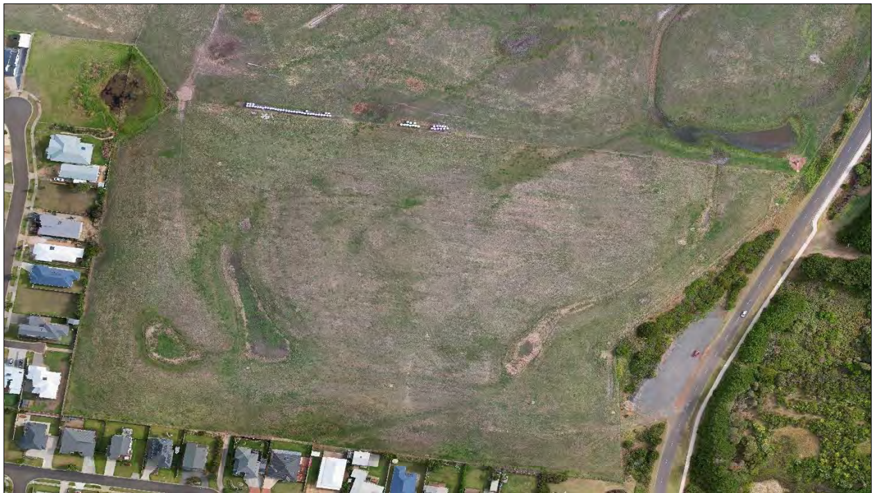
Figure 5 – Existing distribution of within-site modified soakage areas and adjoining roadside regrowth coastal heath vegetation.
