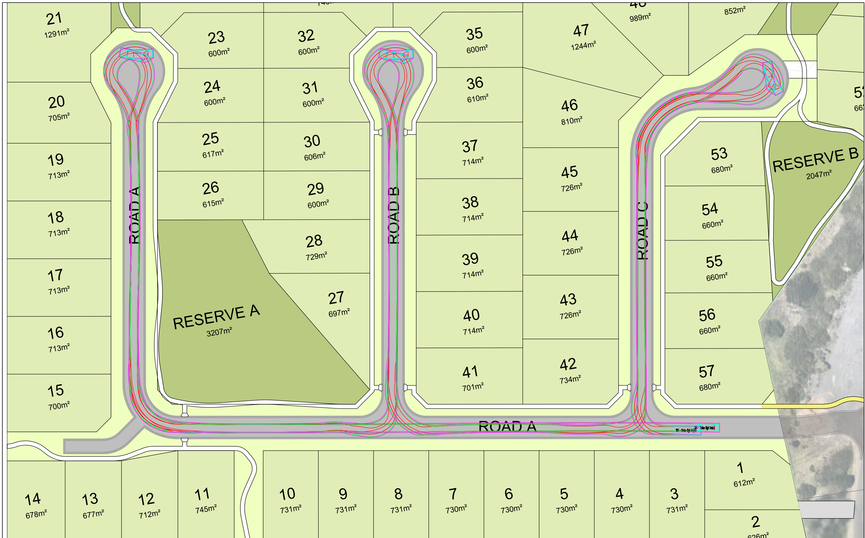
Swept Path Diagram Prepared using AutoDesk Vehicle Tracking v23
