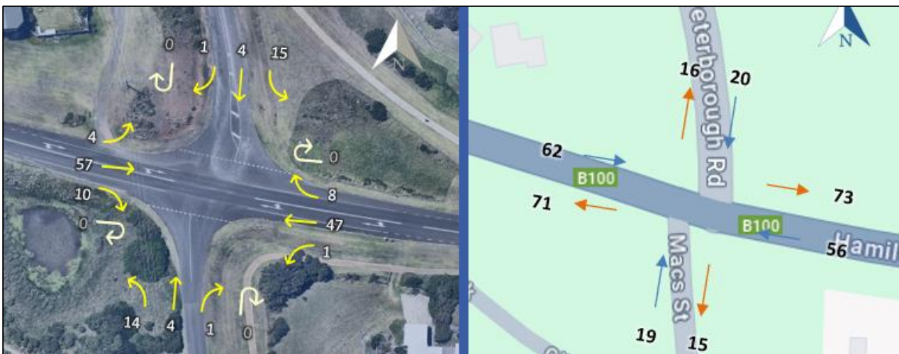
Figure 10: Anticipated AM Peak Hour of Old Peterborough Rd / Great Ocean Rd/ Macs St
