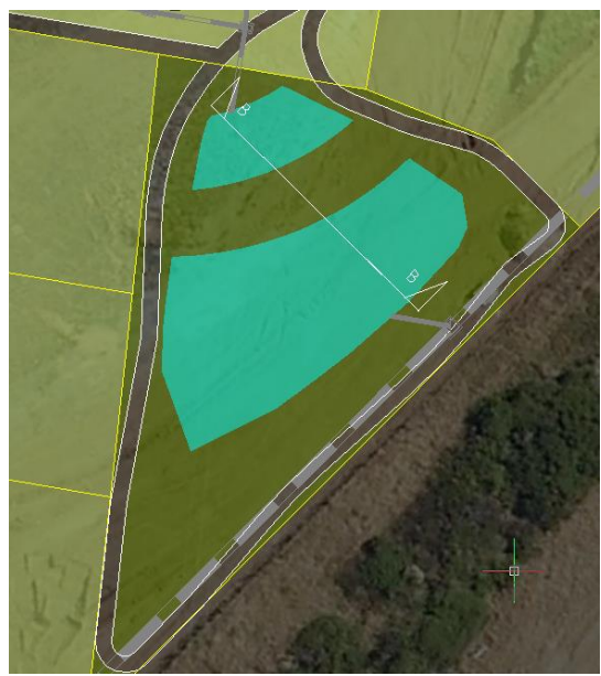
Figure 6 - East Sedimentation and Detention Basin
