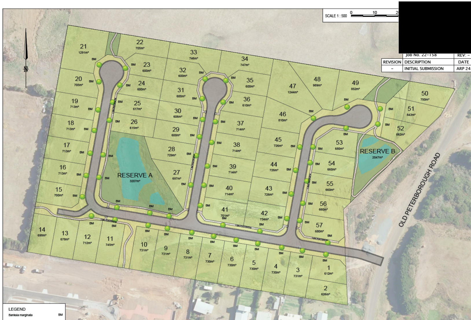
Figure 1 - Subdivision Plan - showing lot layout, concept street trees, reserve areas with pedestrian connections
