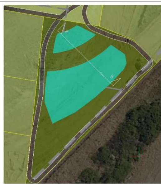
Figure 6 - East Sedimentation and Detention Basin
